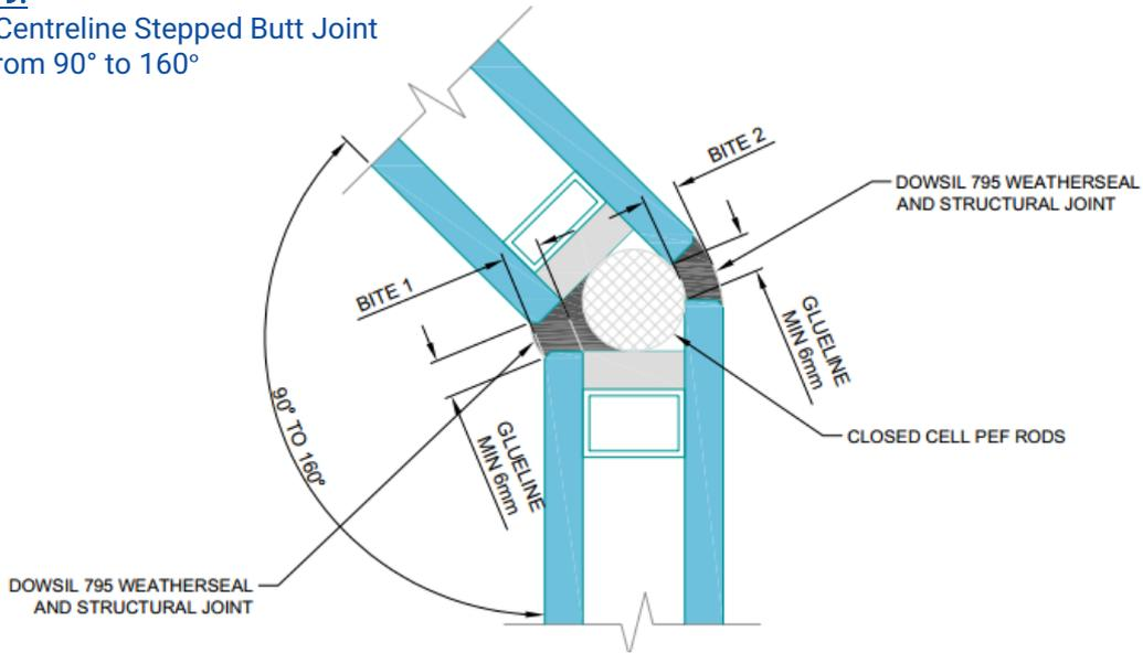
For an IGU with a 160° to 180° degree silicone butt joint, much like the single glazed version there is no support gained from the silicone joint. The IGU's must be designed as two edge supported. Unlike two edge supported monolithic glass which has a deflection limit of span/60mm, two edge supported IGU's have a deflection limit of span/150mm. This often requires thicker glass which can often result in a IGU make-up which is not commercially viable.
