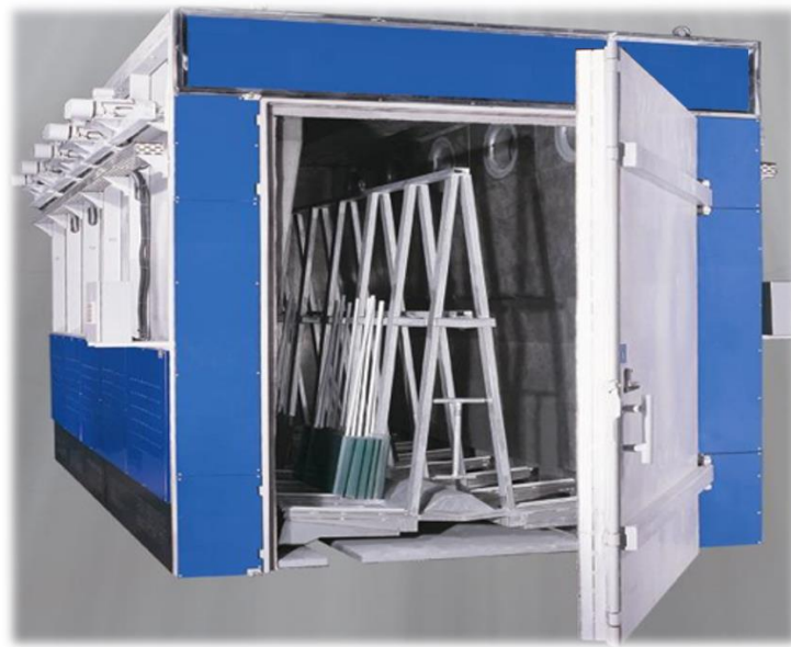
Image 3: Heat Soak Chamber
