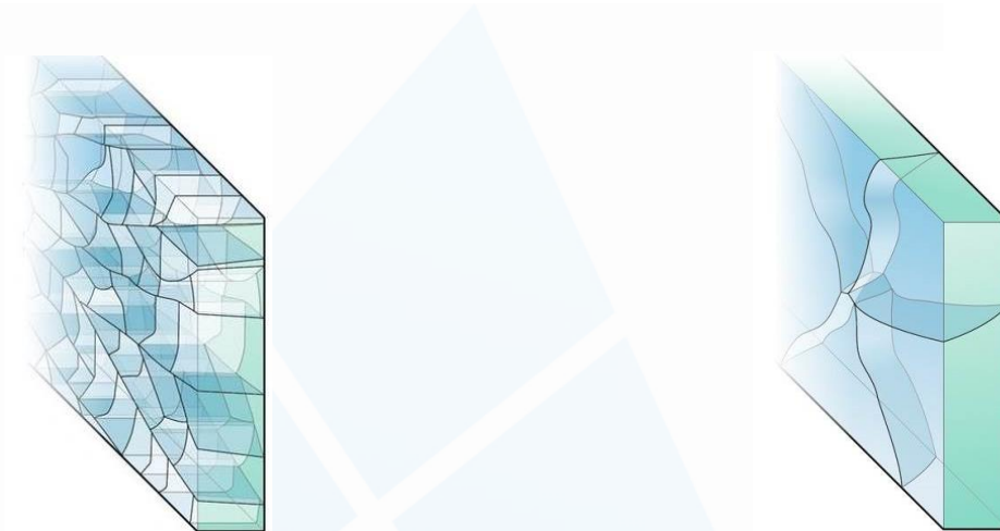
Image 1: Toughened glass break pattern
