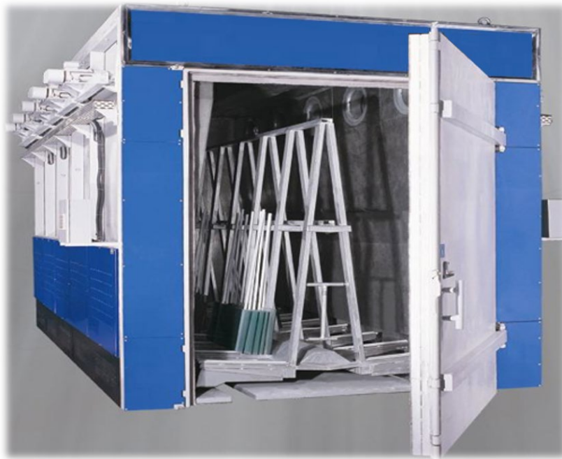
Image 3: Heat Soak Chamber
